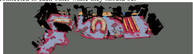
Figure 4: Navigable space represented in a NavMesh
